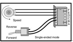
A spare battery - connection is present in case you wish to fit a manual override switch. The diagram shows how a 3 position switch can be used to give release - brake - normal.
