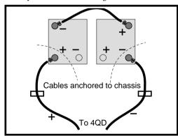
Battery leads are clamped to the vehicle's chassis in such a way that the positive lead can only reach the positive terminal, and then only if the battery is fitted the correct way round in the vehicle.
