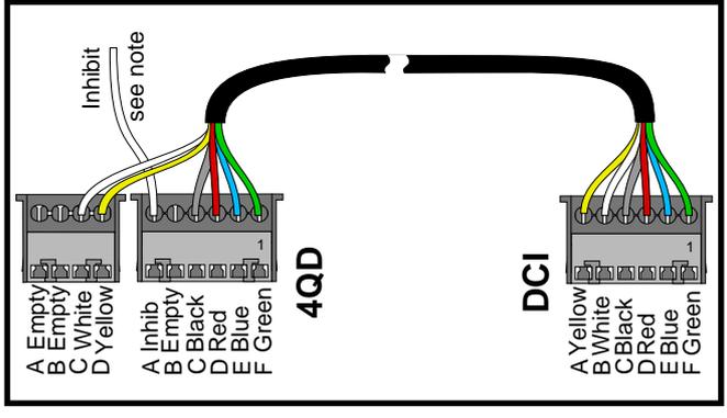
The link lead must be modified as shown above, so that the DCI draws its power off the 24v controller power via the yellow wire. Using the white and yellow wire as above means the DCI ignition must be linked as normal.
