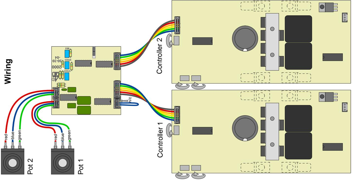
The diagram shows the wiring between interface and controllers.
