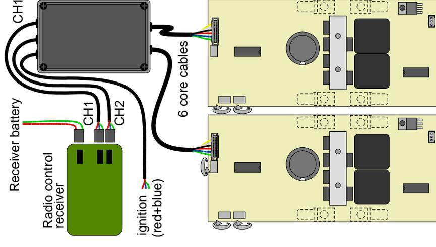
Note that the Interface derives its power from the host controller's pot top (output pins D) connections. The unit will not operate if there is no power to the controllers or if the Ignition connection is not made.
